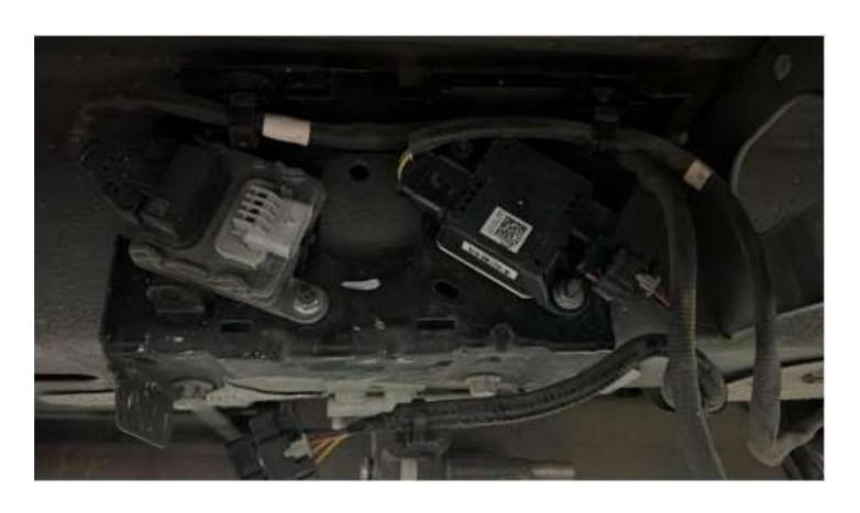
Pull out PM sensor and downstream NOX sensor
